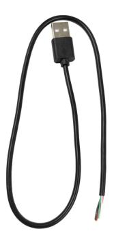
Solder the JWPF crimped wires on the bare USB-A cables.
