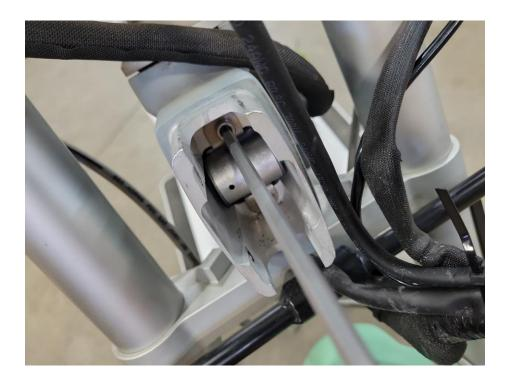
3. Install the new lock cylinder in the same position. Apply Loctite to the securing 5mm bolts
