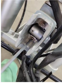
4. Make sure to bundle up the wiring and ensure not to pinch them as you reinstall the front end of the frame. Once the front cap of the frame is in place, reapply Loctite to the 4 securing T20
