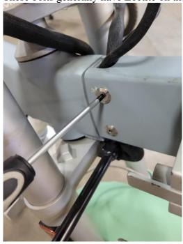
2. Remove the two securing bolts of the steering lock using a 5mm Allen wrench. These bolts generally have Loctite on them, so they can be a bit tight.
