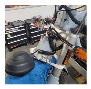
Step 3: Follow the cable from the handlebar switch to where it connects to the bike's main harness. Disconnect this connection. TIP: This connection can be a bit stiff. Be sure to dis-engage the securing clip with your thumb while unplugging the connection.
