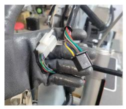
Step 4: Using a Phillip's head screwdriver, remove the 2 securing screws on the handlebar switch. The handlebar switch will then come off completely.
