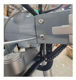
Step 2: Remove the front section of the main beam. Tip: Rest/Secure it on the front fender using a short strap or similar.
