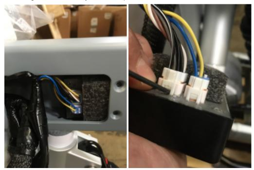
Step 4: Reuse the foam spacers from the old DCDC in order to secure the new DCDC so it will not rattle around in the frame. Reinstall the module and portal plate. Power the bike on and check for functionality of your light system.
