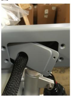
Step 3: The cables will be connected to the DC/DC module in the rear accessory arm at the back - pull gently and reveal the 2 connections. It may be easiest to disconnect these in the bike for easiest removal. In this example I found it easy to remove while still connected. To do this, using a 2mm allen key can be helpful.
