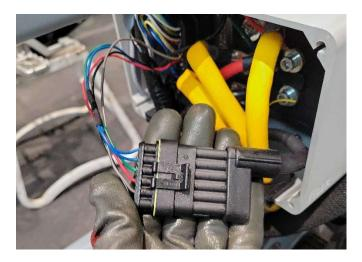
Step 4: Disengage the securing clip of the connector and unplug it. Inspect the pins and associated terminals on the connection. Make sure that nothing looks bent or damaged (very unlikely).
