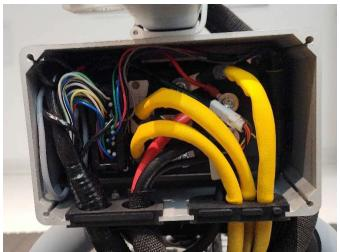
Step 3: Follow the black cable running from the motor into the controller box to locate and identify the motor sensor connection.
