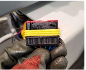
Step 6: If any moisture is observed, we will want to let this connection dry out thoroughly before plugging it back in. Tip: Using compressed air can help get the connector dry faster.
