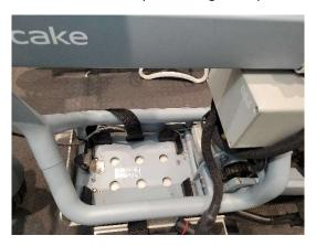
Step 2: Using a Torx T25 bit/driver, remove the 4 securing bolts on the front of the controller box lid. With the lid removed, we will have visibility and access into the controller box. We want to make sure the inside of the controller box is free of any moisture and debris.
