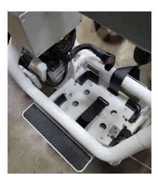
2. Using a Torx T25 bit, remove the 4 securing bolts for the controller lid
