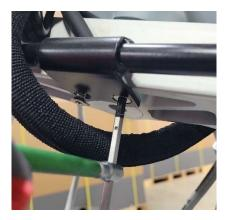
Step 11: Slide the large cable harness back underneath the upper fork assembly.
