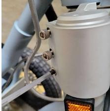
Step 13: Using a 5mm Allen Wrench, re-install the 2 brake cable guides. Ensure that the brake hose is routed through the guide. Apply a drop of Loctite 243 to the bolt threads and tighten to roughly 10Nm.
