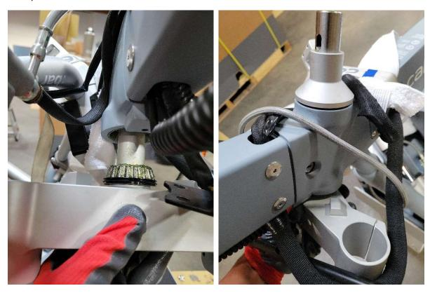
Step 9: Slide the handlebars back onto the steer tube. Using an 8mm Allen Wrench, re-install the top steering bolt. Hand tighten only for now. This bolt will hold the assembly together while we re-install the remaining pieces.
