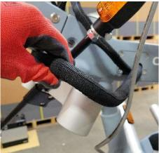
Step 6: Using a 5mm Allen Wrench, loosen the 2 pinch bolts on the stem. You do not need to remove them completely, just loose.
