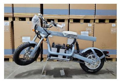
Step 2: Using a 5mm Allen Wrench, remove the 2 brake cable guides.
