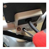
Step 15: Make sure the front wheel and the handlebar are perfectly aligned. When the handlebar is straight, use an 8mm Allen Wrench and tighten the top steering bolt to roughly 15Nm. Then, using a 5mm Allen Wrench, tighten the two pinch bolts to roughly 10Nm. Lastly, release the pressure from the top steering bolt and then tighten it again to roughly 10Nm. **Helpful video found HERE** – **watching is recommended.**
