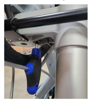
Step 3: Using a Torx T30 Driver/Key, remove the 2 securing bolts for the front turn signal assembly.
