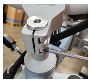
Step 7: Using a 5mm Allen Wrench, remove the bolt located in the front of the stem.
