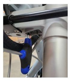
Step 14: Align the handlebars straight with the front wheel. Using a 5mm Allen Wrench, re-install the bolt located in the front of the stem. Tighten to roughly 10Nm.
