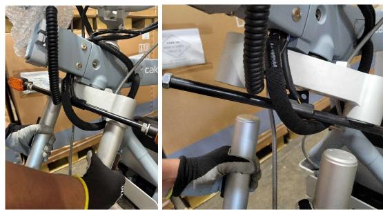
Step 5: Slide the large cable harness out from underneath the upper fork assembly.
