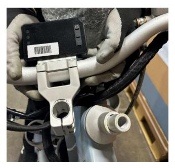
Step 8C: While the 2<sup>nd</sup> person holds the handlebars, slide the original steering column out and the new one in. Take note of the upper bearing, o-ring, and top spacer. They should remain in place.
