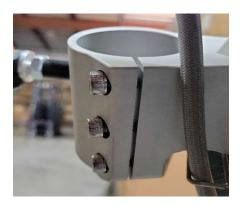
Step 12B: Slide the forks back up into the fork assembly. Make sure that the brake lines are routed behind the fork assembly first. Slide the forks up until the top sits above the assembly just 7-10mm. Rotate the fork so the reflector is facing outward.
