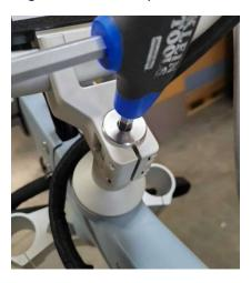
Step 8B: Slide the handlebars up and off the steering tube. Have a 2<sup>nd</sup> person help and hold the handlebars.
