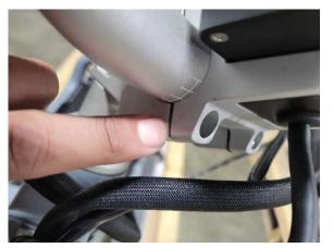
Step 9: Reinstall the large 8mm top cap. Tighten this to 15Nm using a torque wrench.
