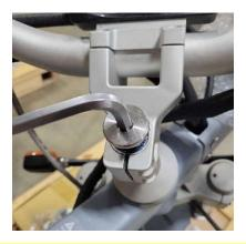
Apply Loctite to the removed hardware (they will be re-used)
