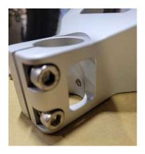
Step 5: Remove the four 5mm bolts that secure the display screen. The handlebars and display screen will be free now and **should be held carefully by a 2**<sup>nd</sup> **individual.**
