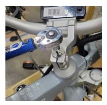
Step 10: Ensure that the handlebars are perfectly straight and aligned with the front wheel. Tighten the two 5mm pinch bolts to 10Nm.
