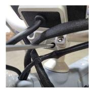
Step 8A: Reinstall the handlebar and display screen. Tighten the four 5mm securing bolts to 10Nm. Tighten them in a "star" pattern (tightening them each in small intervals, rotating between them).
