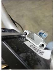
Step 8B: Make sure the handlebar is centered (left to right) and angled to the -5 degrees angle mark.
