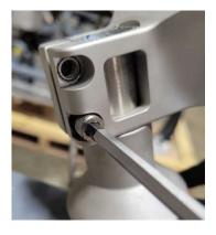
Step 2: Remove the 5mm safety bolt in the front of the stem.
