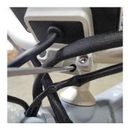
Step 3: Remove the large 8mm stem top cap.
