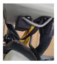
Step 2: Using a Torx T25 bit/driver, remove the 4 securing bolts of the controller box.
