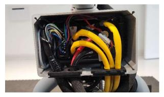
Step 3: Using the Torx T20 and a 7mm wrench, remove the 2 securing bolts for the module.
