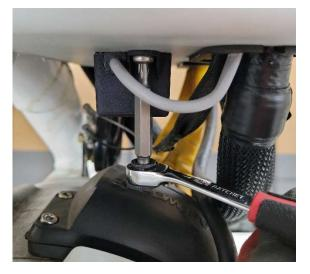
Step 4: Unplug the connection of the module the bikes wiring harness.
