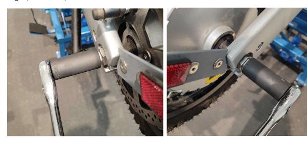
Step 3: Using a 6mm Allen wrench, remove the 2 X 6mm bolts that secure the rear fender bracket
