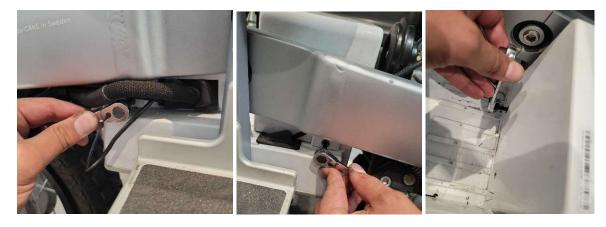
Step 7: Partially remove the controller box cover. Rest it in the battery tray, as there is no need to disconnect the connections running from it to the controller.
