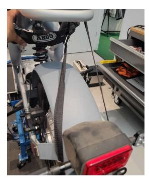
Step 5: There are 3 power cable guides that secure the main power cord to the inside of the swingarm. Using a Torx T25, remove the 3 cable guides. Tip: Sometimes the cable guide closest to the rear hub can be hard to access. Waiting to remove this cable guide until you can pull the rear wheel back and out of the way can be a work-around for this.
