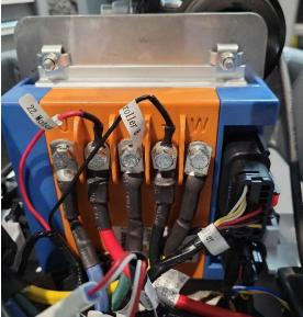
Step 8: Using a 8mm socket, remove the 3 phase cable connections to the controller.
