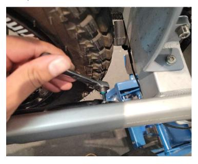
Step 6: Using a Torx T25, remove the 4 securing bolts for the controller box cover. Tip: The bolt on the right side of the cover can be tricky to access, as it is behind the main power cable to the rear wheel (photo below of its location).
