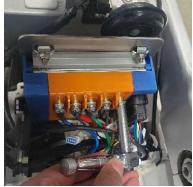
Step 9: Unplug the 6 pin plastic connection on the motor power cable.
