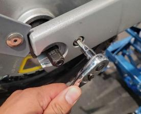
Step 4: Using a Torx T20, remove the 4 securing bolts for the rear fender.
