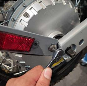
Tip: If you have a short strap, supporting the rear fender can help keep it out of the way during the wheel removal.
