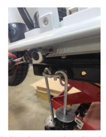
6. Remove 3 X T25 screws on left side plastic body work. Remove the Bodywork piece.
