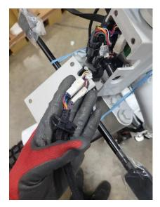
5. Remove the ride side foot plate by removing the 4 X T45 bolts
