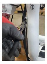
3. Remove the 4 X T45 bolts that secure the headlight assembly. Use a strap, rubber band, or similar to suspend the headlight assembly. We want to avoid letting the headlight hang by the wires.
