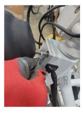
4. Disconnect the 2 white JST connections coming from the handlebar assembly. Take note (or photo) of how the cables and plugs are packed into this area, as it will be helpful upon re-install.
