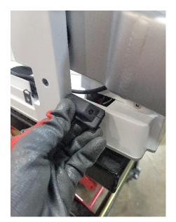
7. Cut the cable ties beneath the plastic bodywork
