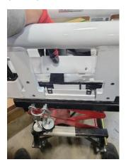
7. FOR REINSTALLATION: make sure to get the two rubber gromets in place, as it will help with the reinstallation of the plastic bodywork piece.
