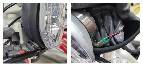
Step 2: Firmly pull out to disconnect these 2 connections. Push the cables out of the rubber hood.
