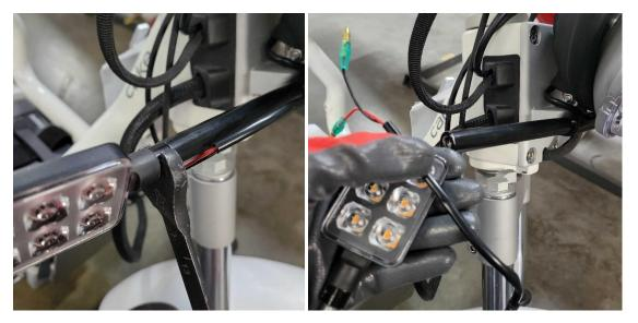
Step 4: Begin installing the new Turnsignal. Push the new Turnsignal cables through the assembly, and into the rubber hood.
