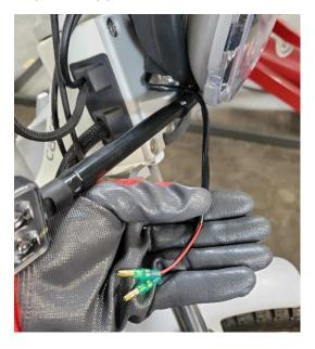
Step 3: Loosen the 13mm nut on the Turnsignal all the way, until the Turnsignal can be removed, and the cables pulled out of the assembly.
