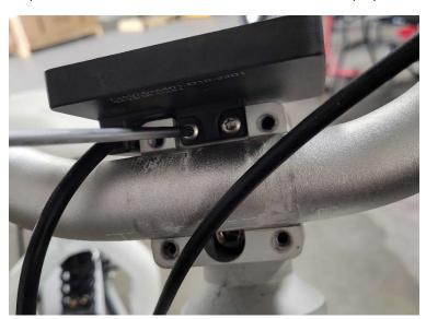
Step 4: Follow the display cable and disconnect the main connection.
