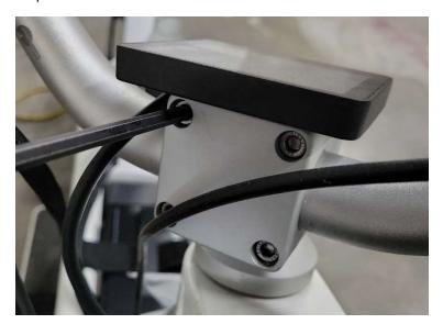
Step 3: Remove the two T20 bolts that secure the display to the handlebar stem.
