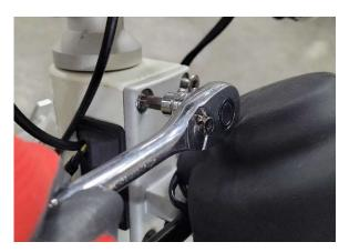
To angle the headlight, gently loosen the securing 5mm bolt until the headlight can be tilted forward.
