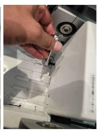
Step 3: Remove the controller cover.
