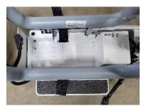
Step 2: Using a T25, remove the 4 securing bolts for the controller cover. A small note - The bolt on the right side of the cover can be tricky to access, as it is behind the main power cable to the rear wheel (photo below of its location).
