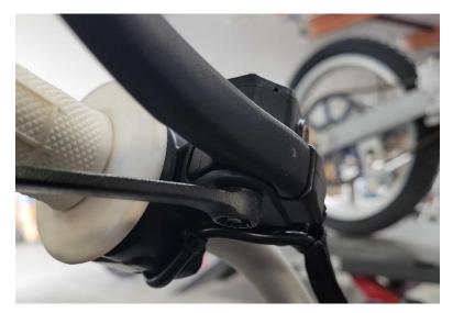
Step 2: Push the securing bolt up and out of the brake assembly. The lever will come off the assembly once removed.
