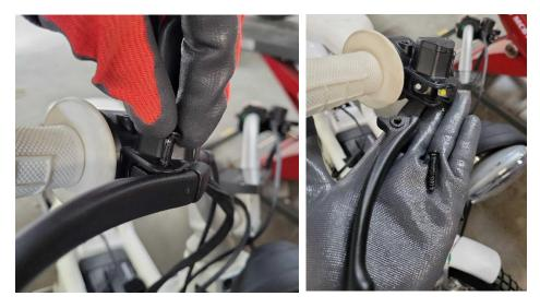
Step 3: Insert the new lever into the assembly and put the securing bolt through the assembly.
