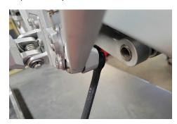
Step 2: Using a T40 key/bit, loosen the main bolt that the sidestand rotates on. Loosening the bolt just a ¼ turn may be all that is needed to allow the sidestand to move freely, and spring up into the resting position automatically.
