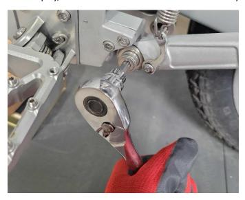
Step 3: With the securing bolt in the correct position, hold it in place using the t40 bit/key and tighten the 13mm locknut on the backside of the assembly to "lock" its position.
