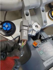
Step 3: Using a 5mm Allen Wrench, remove the 4 securing bolts for the dashboard to remove it completely. Caution - The handlebars will be loose after this!
