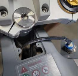
Step 2: Follow the cable coming off the back of the display unit to locate where it connects to the bike's main harness. Unplug.
