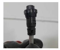
Step 7: Using either the same needle nose pliers, or a pair that is slightly larger, firmly re-crimp the 2 tabs onto the cable. Crimp this firmly, as it is these 2 tabs that will prevent the terminal from being pushed down in the future.
