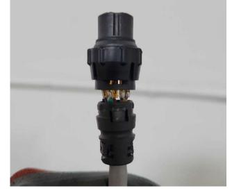
Step 5: Identify which terminal needs to be pushed back into place. Using a pair of precision needle nose pliers, push the terminal back up until it is visible and the same height as the others.
