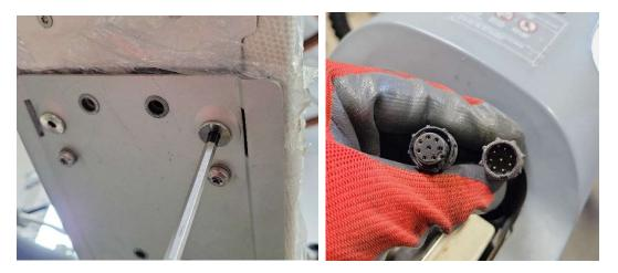
Step 2: Pull back/down the exterior rubber cover of the connection.
