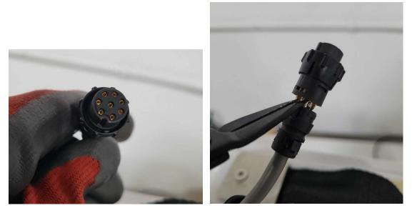
Step 6: With the terminal back into the correct position, we can then slide the lower half of the connection back into place, engaging the 2 securing clips again.
