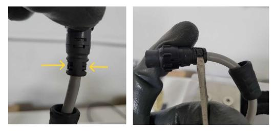
Step 4: Using the same small flat head screwdriver, we will then disengage the 2 securing clips that hold the connection assembly together. With these 2 securing clips disengaged, the connector can be pulled open, sliding the crimping side on the connector tube the cable. (Note – in the below photos, the crimping tabs have already been loosened)
