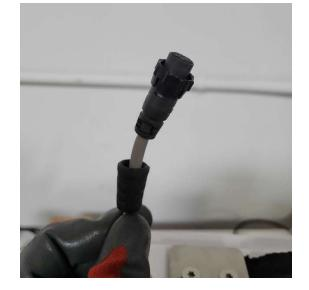
Step 3: With this area visible, we can see that there are 2 tabs that are crimped during assembly to hold the terminals in place. We need to very gently relieve some of the crimping pressure by using a small flat head screwdriver. Do not unfold the tabs completely, just gently pry them back ~1mm.
