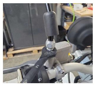
Step 2: Using a 17mm wrench, loosen the "lock-nut" which will allow the mirror to rotate freely. We do not want the 14mm to loosen during this step, so you may need to hold the securing 14mm in place while you loosen the 17mm.
