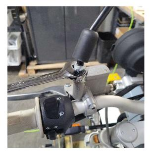
Step 3: While sitting on the bike, adjust the mirror position to your liking. Hold the mirror in place, and tighten the 17mm locknut. This will lock the mirror in that position.
