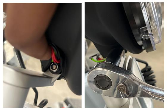
Step 2B: After you have the lock nut removed, use a 5mm key/bit to loosen the bolt and adjust your headlight to desired position. Once in position, tighten down the 5mm bolt as tight as possible
