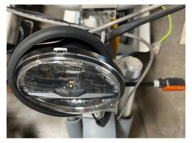
Step 2: Using a 10mm socket, remove the securing lock nut for the headlight. A small note - The nut on the left side of the cover can be tricky to see, as it is underneath the rubber bumper (photo below of its location).
