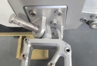
Step 3: Firmly insert the spring into the footpeg. The securing bolt should not interfere when pushing the spring into place, and the spring should remain in place after it is inserted.
