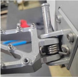
Step 4: With the spring in place, begin to tap the securing bolt all the way through the spring and footpeg with a rubber mallet. You may have to adjust the resting position of the spring to ensure that it lines up with the bolt prior to tapping it through with the mallet.
