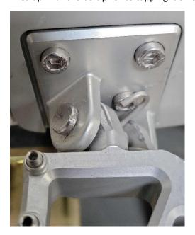
Step 5: With the securing bolt in place, install the washer and cotter pin. Bend the ends of the cotter pin to ensure the securing bolt will not come out during normal use.
