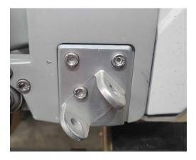
Step 2: Lightly get the footpeg into place. Insert the securing bolt partially, so it holds the footpeg in place, but does not interfere with the insertion of the spring.
