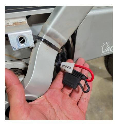
Once you locate the fuse, pull back the rubber cover and remove it. It will have a number "3" on it. Identify whether the fuse is still good. See graphic below.
